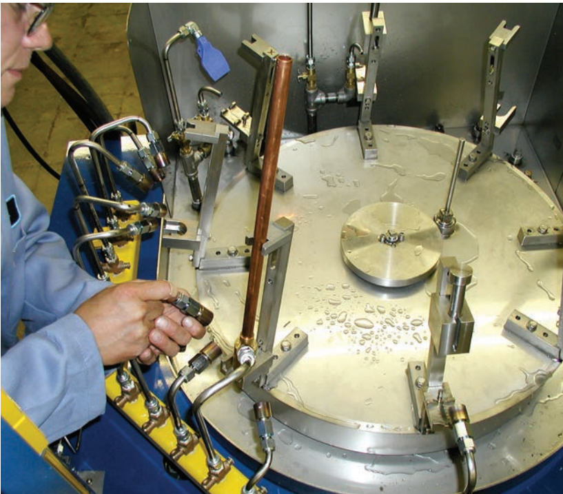
Top: Prototype tooling is mounted on a lab machine to determine paste application method, heat pattern, and production rate achievable. Middle: Feasibility testing parameters are designed into the final machine production fixture to maintain brazed/soldered assembly specifications. Bottom: Service technician installs brazing machine and instructs personnel in your plant.
