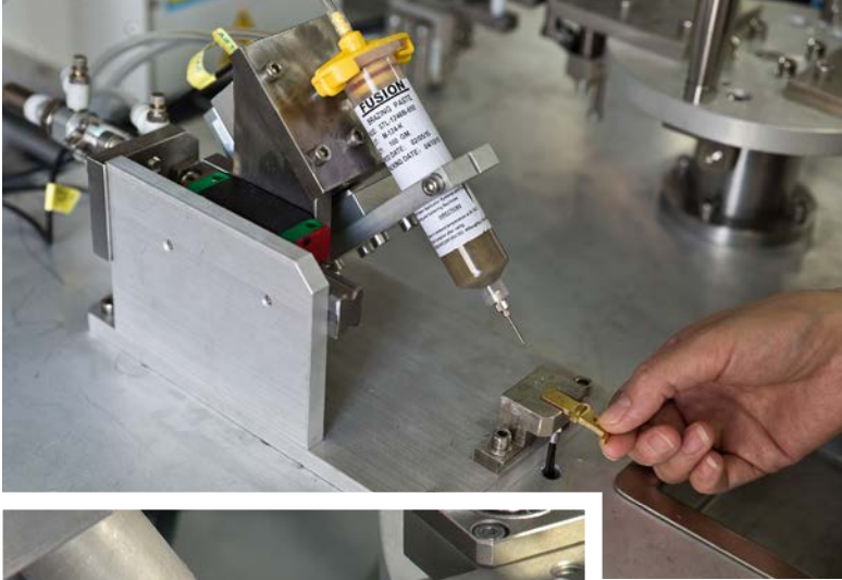
Silver paste dispensed from cartridge onto electrical contact base prior to induction heating.
